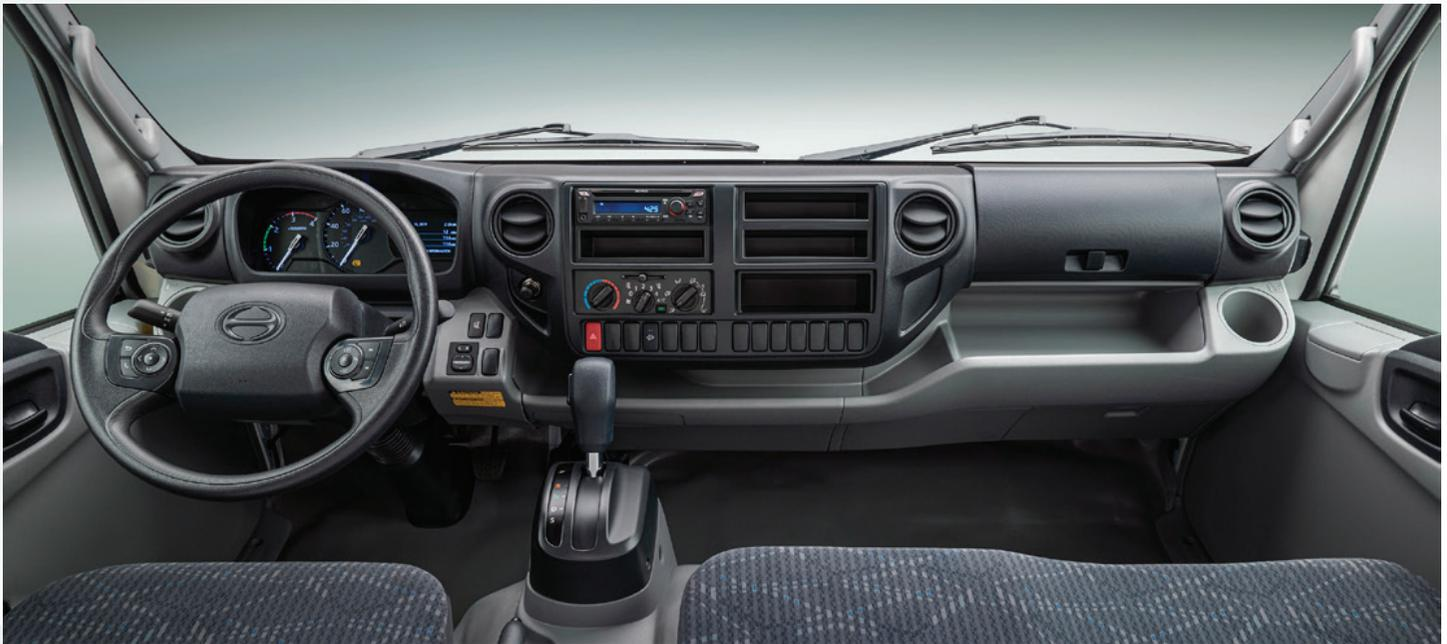
NEW interior design equals more functionality! A new gauge cluster featuring a 4.2" LCD multi-information display for easier vehicle monitoring and a new Aisin 6-speed HD automatic transmission with a gear hold feature, especially useful in steep incline situations.
