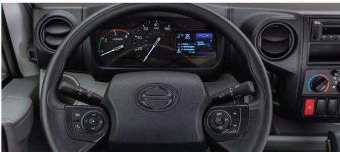
New steering wheel with interaction controls such as cruise control to reduce time off the wheel.
